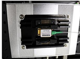
1550nm PM SLD Laser diode
