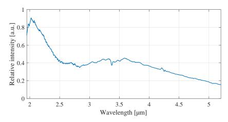
Spectrum of emitted light from L1280 between 1.95  $\mu m$  and 5.2  $\mu m$ . The light source does not imitate a black-body emitter perfectly, but it resembles a black-body emitter with a temperature of approx. 1200 °C.
